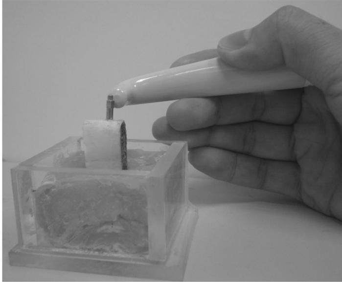
Figure 1. Experimental measurement set-up for dental implant–bovine bone structure. The rib bone with a dental implant is inserted into a resin block. An aluminium rod is screwed into the implant and excited by an electromagnetic pulse from the measurement probe.
